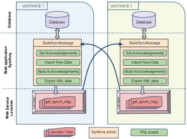
Figure 1 - Overview of the architecture and synchronization
