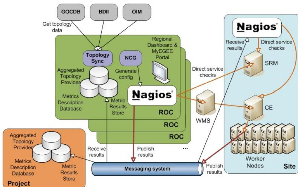
**Figure 5. Architecture of the SAM framework**
