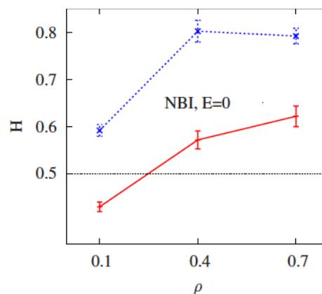
**Fig.3 - Profile of Hurst exponent in plasmas of TJ-II device. A ballistic behaviour is observed for the outer positions.**
