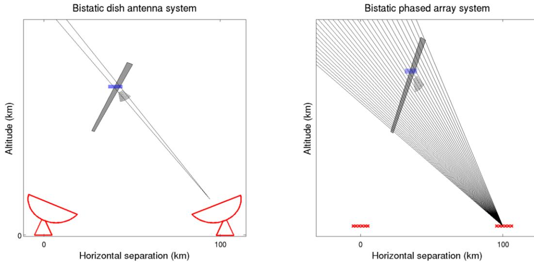
**Fig.1 - This sketch compares bi-static phased array (right) and conventional dish radar (left). (Prepared within the FP7 Preparatory Phase by B. Gustavsson, EISCAT Scientific Association).**
