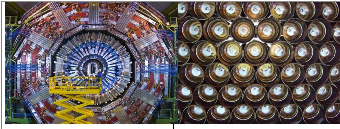
**Left: Transversal view of the CMS detector. Right: A view of the photomultiplier tubes used in the LHCb detector.**
