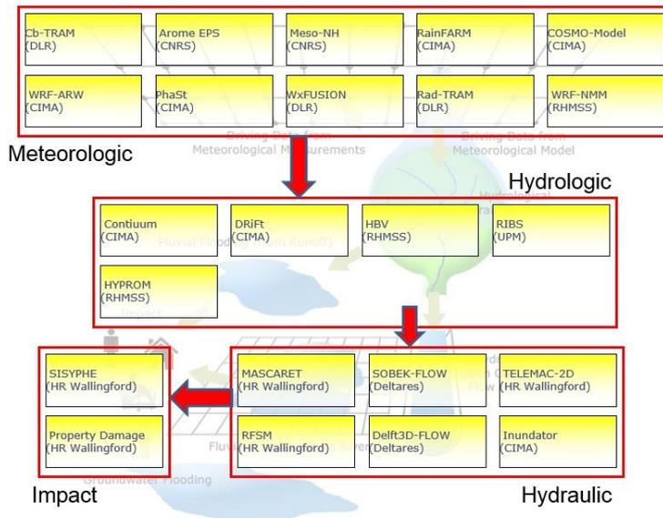
**Fig. 10 - DRIHM models classified in related layer. A workflow may be composed of one model for each level.**
