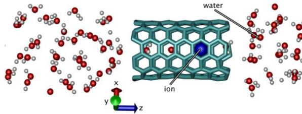
**Fig.2 - Solvated ion flux through an open end carbon nanotube.**
