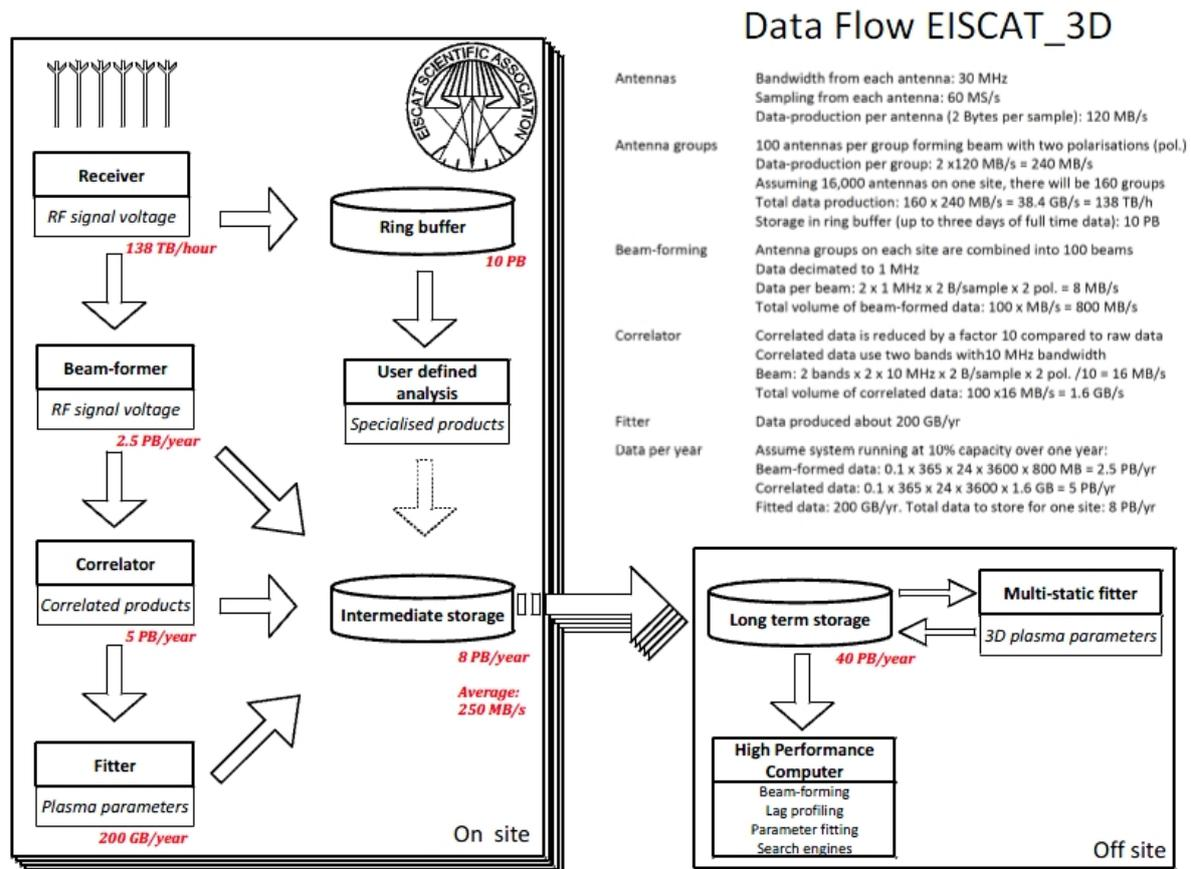
**Fig.2 - The expected maximum data flow for EISCAT\_3D. Figure prepared within the FP7 Preparatory Phase by A. Tjulin, EISCAT Scientific Association.**
