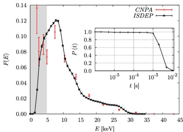
Fig.5 - Comparison of the measured (red points) spectrum of fast ions with the calculated one (black line) in TJ-II. The persistence of ions in the plasma is also plotted in the small chart.
