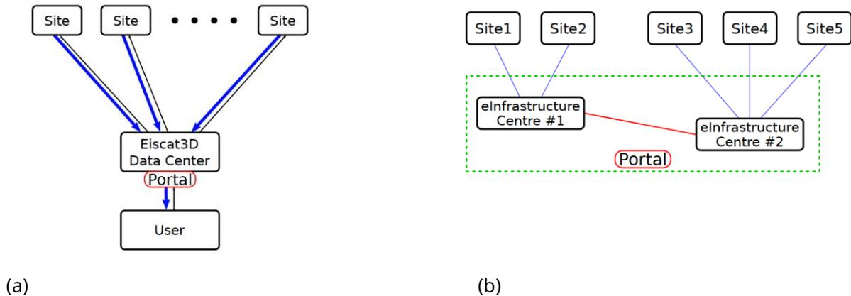
**Fig.3 - The data central (a) and distributed solution for the EISCAT\_3D data centre. The figure is prepared within the FP7 Preparatory Phase by M. Nylén, Physics Department, Umeå University, Sweden and Swedish National Infrastructure for Computing (SNIC).**
