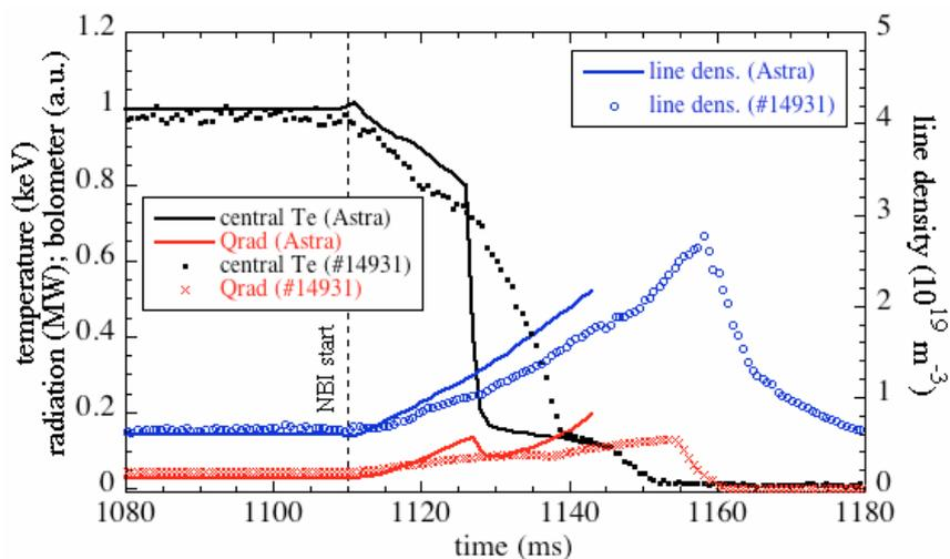
Fig.7- Time evolution of plasma parameters in TJ-II. Continuous lines are calculated, while dotted lines are experimental results.
