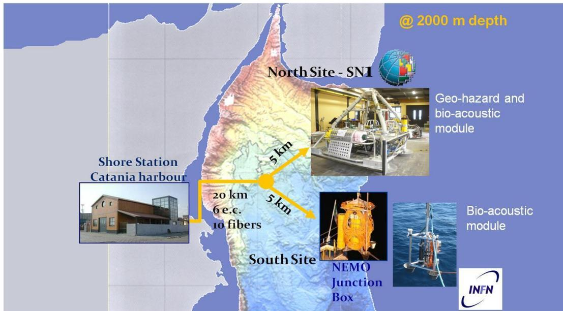
**Fig.3 - The EMSO node offshore Catania**
