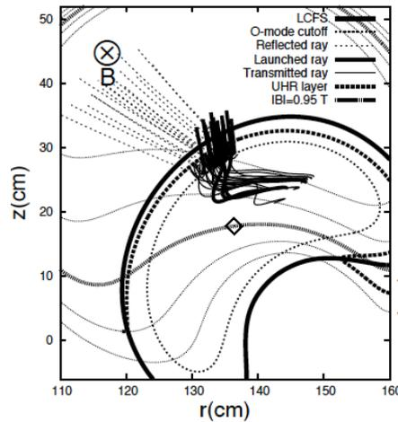
Fig.6 - Rays of microwaves in the TJ-II plasma.
