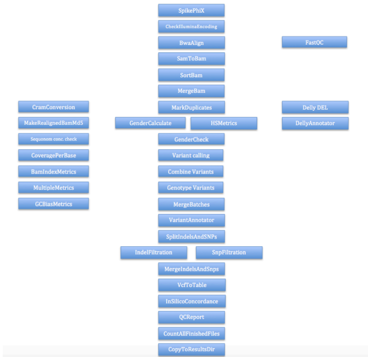
Figure 2: Summary of the NGS_DNA pipeline. Dataflow from top to bottom; parallel tasks are shown next to each other. At various steps the analysis is run split in smaller parallel jobs (not shown), e.g., alignment is parallelised per NGS machine run, variant calling is run for each of the 23 chromosomes separately. An analysis can consist of up to hundreds of samples resulting in a sizeable analysis task.
