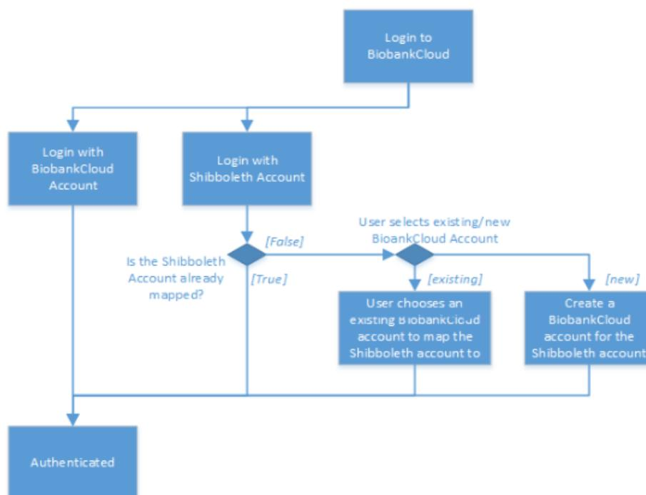
Figure 2. BiobankCloud Login Process with Shibboleth Enabled
