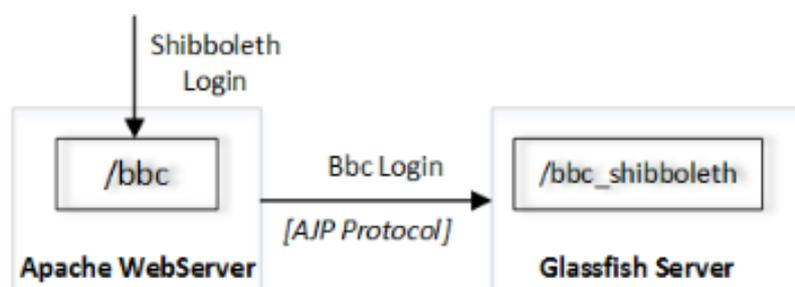
Figure 1. Shibboleth Login to BiobankCloud by fronting the Glassfish Server (running BiobankCloud) with a Apache Server that proxies requests to Glassfish using the AJP Apache module.
