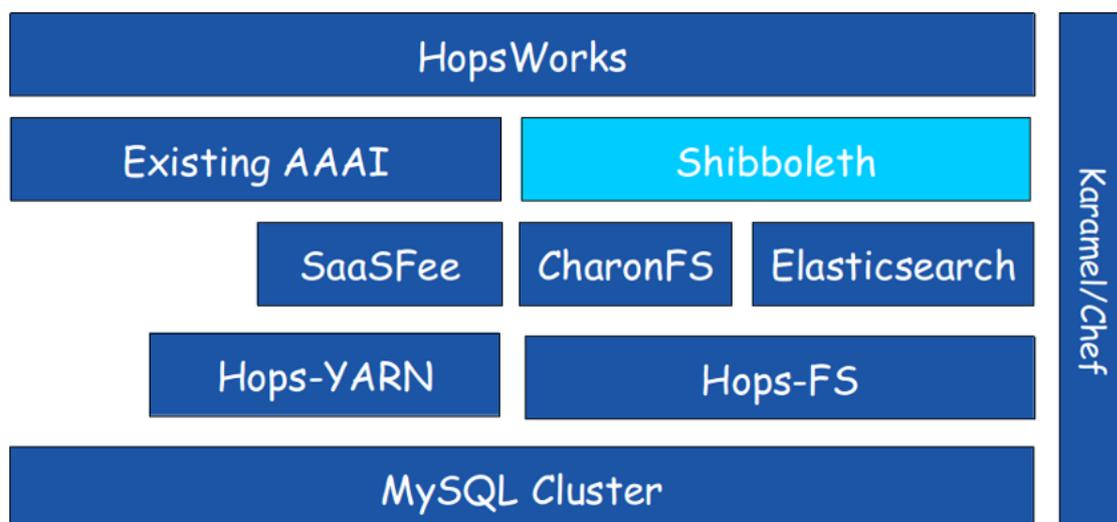
Figure 3. BiobankCloud Architecture with Added support for Shibboleth
