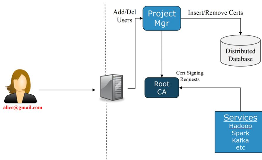
Figure 4. BiobankCloud (Hopsworks) has been extended to provide an X.509 certificate for each project-specific user as well as a host-specific certificate that is shared by services, such as Hadoop YARN, the Hadoop filesystem (HDFS), Spark, and Kafka.
