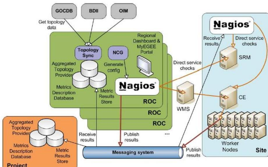
**Figure 1. Configuration of the fully regionalized Nagios-based monitoring infrastructure.**
