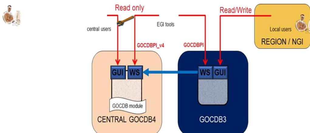
Figure 6. Synchronization between GOCDDB3 and GOCDDB4
