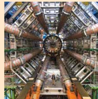
It's no mean feat to accelerate particles around a 27km ring close to the speed of light, then colliding them 800 million times a second. Only one machine in the world is capable of this job – the Large Hadron Collider (LHC), a particle accelerator located 100m underneath the French/Swiss border.
