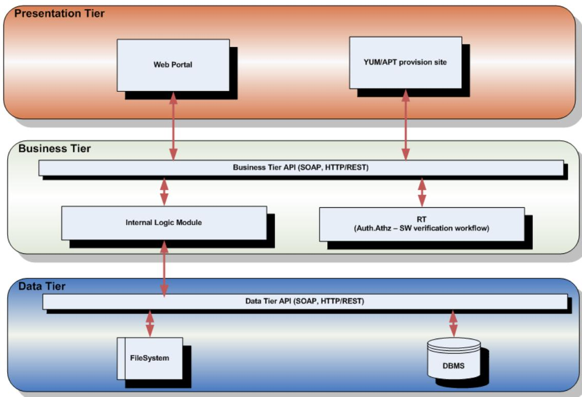
**Figure 3: Three-tier system architecture diagram**
